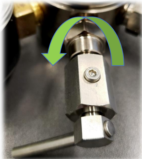
Figure 20b: To open the bleeder and release Air, turn the Valve Nob Counter-Clockwise.
